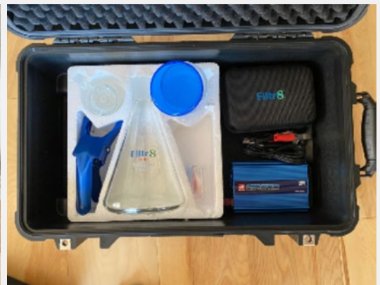
Figure 3. Portable ScavSol™ Injectivity Performance Stimulation (IP 2 Predictive Method); filtration equipment, power inverter for tailgate testing
